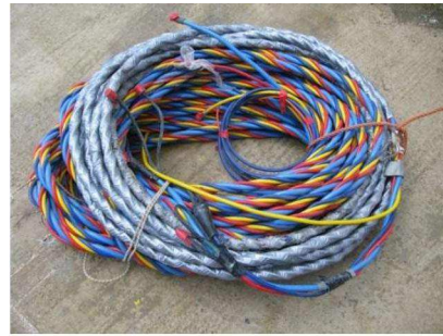
Ombelicale Gas PneumoCom. Video e faro
